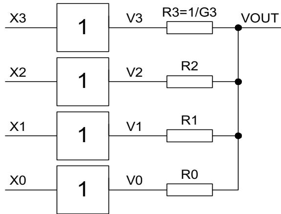
$$(V_3 - V_{OUT})G_3 + \dots + (V_0 - V_{OUT})G_0 = 0$$
