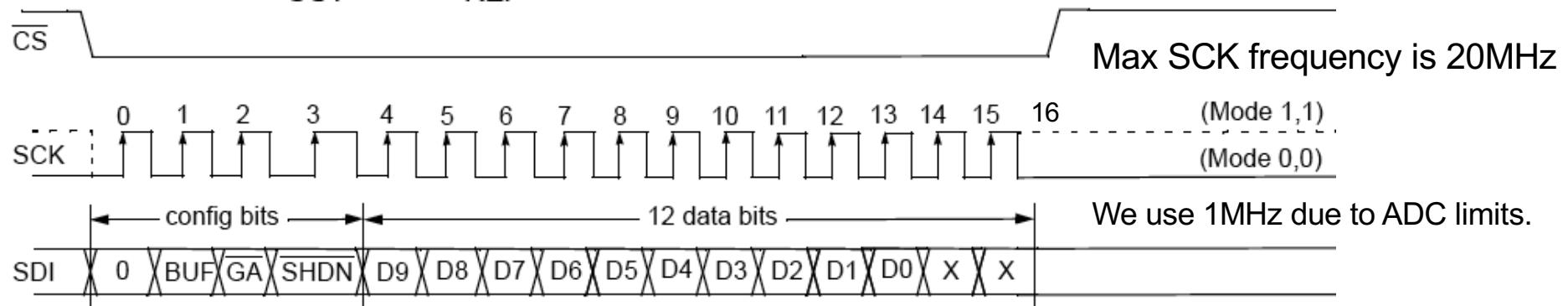
**LDAC** If  $\overline{LDAC}$  is tied to ground,  $V_{OUT}$  is updated on rising edge of  $\overline{CS}$ .
